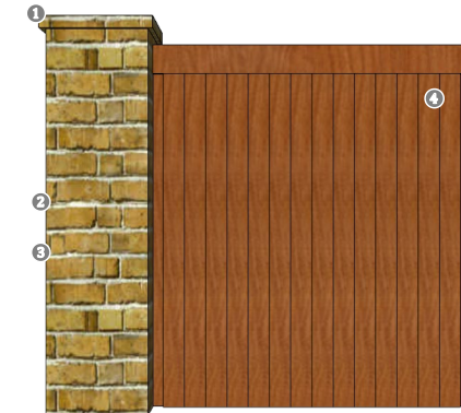
1: Rowlock Cap; 2: Running Bond; 3: 3/8" Tooled Joints (Typical); 4: Wrought Iron or Board-On-Board Wood Fence.
